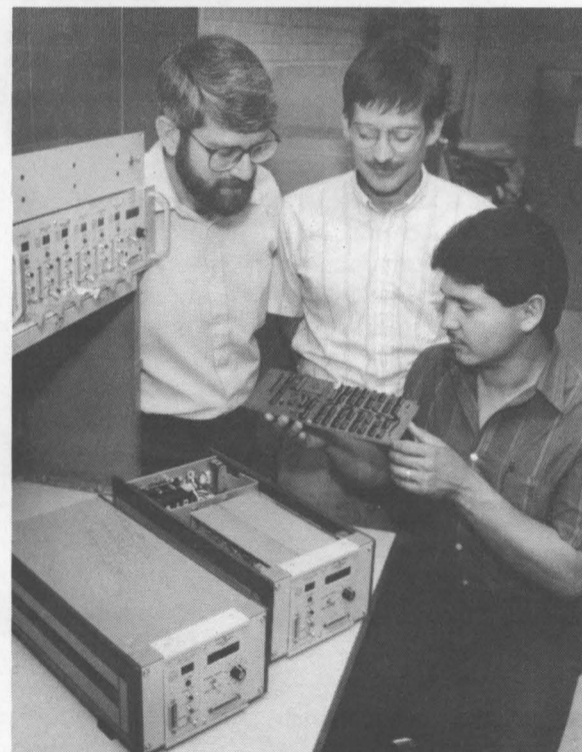
CRYPTOGRAPHIC SYNCHRONIZATION loss detector was developed by (from left) Lyndon Pierson, Tom Pratt, and Joseph Maestas (all 1934). The two boxes on the bench are the version that won an R&D 100 award; Joseph is holding a newer, smaller, faster version that's in the prototype stage.
